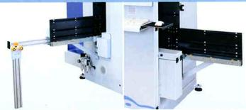
Mechanical support via roller conveyor in the loading- and removal area of the machine.
