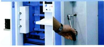
Easy adjusting to different workpiece thicknesses. The required workpiece thickness can be controlled optically via monitor.
