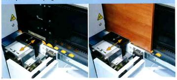
Easy adjustment of the clamping device (manually) to the workpiece thickness (clamping device stroke 6 mm). For differences in the workpiece thickness of up to 6 mm it is not necessary to manually adjust the clamping device.
