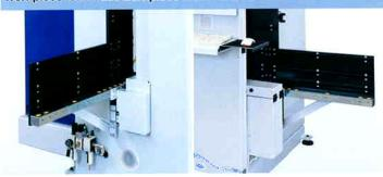
Mechanical support via roller conveyor in the loading- and removal area of the machine.
