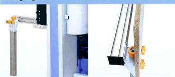
Extension of the working length to 3050 mm incl. roller conveyor
